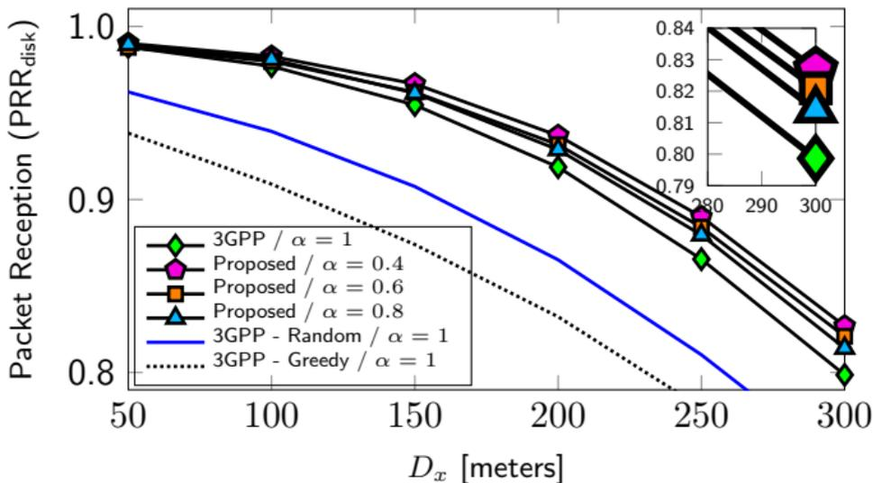
Figure 6: PRR<sub>disk</sub> for an urban scenario with  $p_{keep} = 0$
