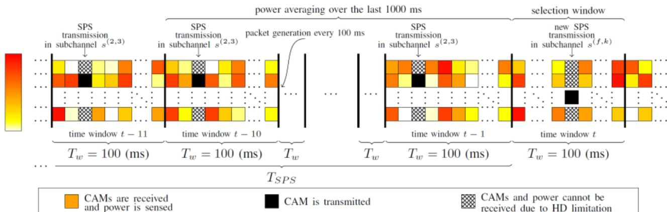
Figure 4: Scheme with joint SPS scheduling and random retransmissions
