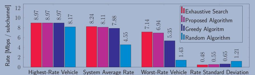
Figure 4: Data rate per vehicle
