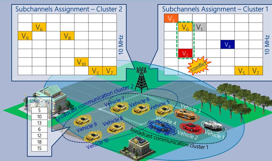
Figure 1: Broadcast communications via sidelink V2V mode-3
